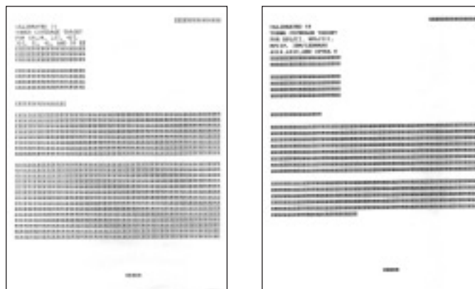
An example of how 5% coverage might look in a business letter format. The left page was printed on an EX printer and the right page printed on an SX printer
